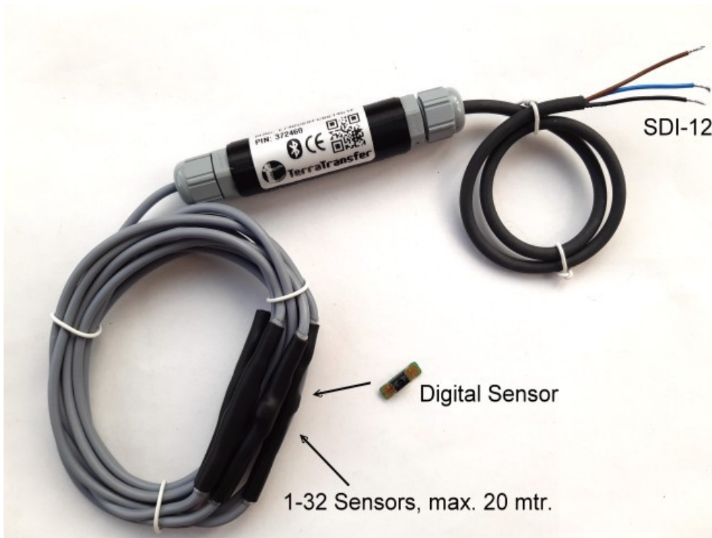
Low cost Thermistor String with 5 sensors. Important: IP64 (not waterproof)
