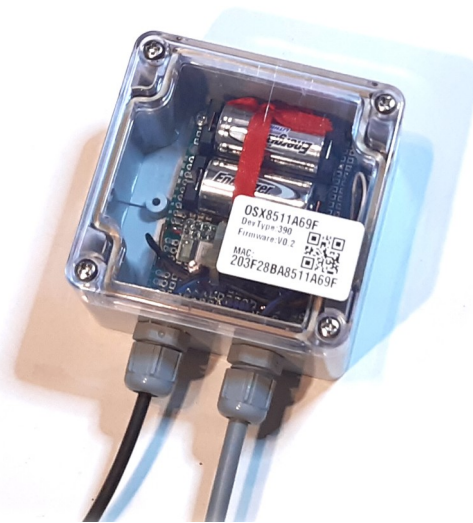
Modbus to SDI-12 / Bluetooth LE Converter (Version B with 2 internal CR123A Batteries)
