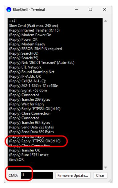
A transfer can be started manually with 'i' (default), 'i1' (more text) or 'i3' (more text and extra long network search, for tests). The text "FTPSSL:OK" shows that the connection to the FTP server was successful.
